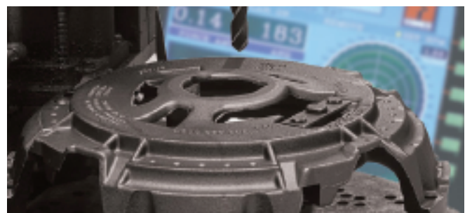
After machining, covers are computer balanced to within 1/4 of an ounce.
