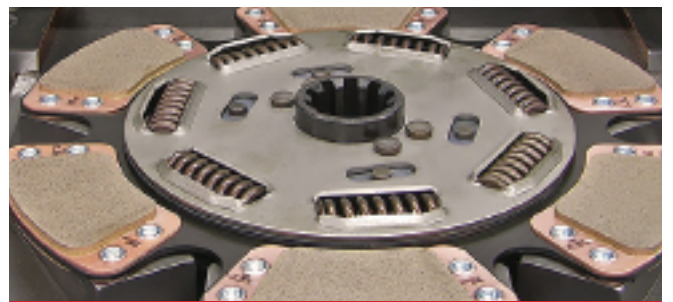
Buttons are pressed in a one-step operation.
